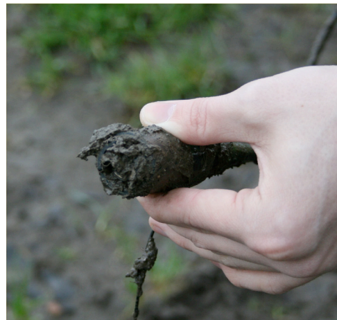
2. The mud will not cause damage to the expanded beam insert. A butt-contact connector would almost certainly already be destroyed in this state.
