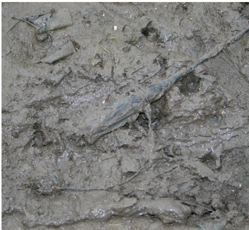
1. Plug connector immersed in mud. The connector is fully sealed even without the dust cap fitted.
